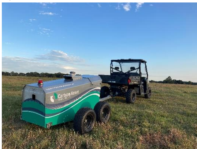
Figure 4: Device for in-situ measurement of soil carbon based on inelastic neutron scattering.
